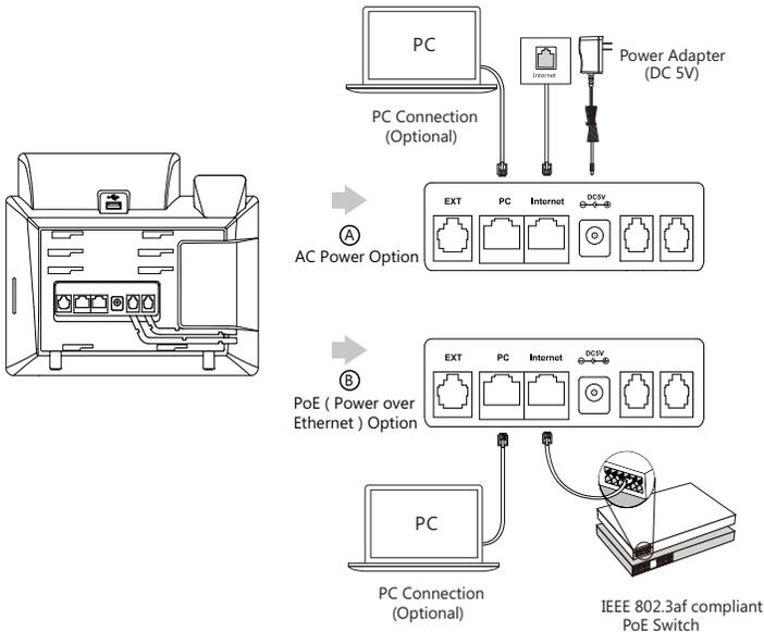
**Note:** The IP phone should be used with ZULTYS original power adapter (5V/2A) only. The use of a third-party power adapter may cause damage to the phone. If you are connecting a PC to your phone, we recommend that you use the Ethernet cable provided by ZULTYS.
