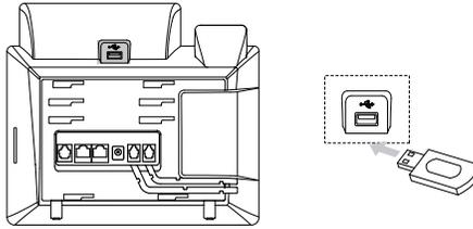
**Note:** The USB port can be used to connect a Bluetooth USB dongle or Wi-Fi USB dongle. The Bluetooth USB dongle and Wi-Fi USB dongle are optional and purchased separately.
