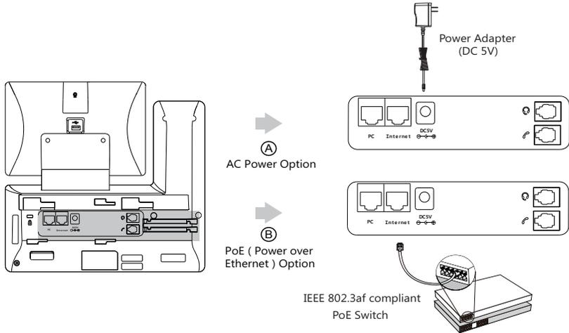
Note: The IP phone should be used with a ZULTYS original power adapter (5V/2A) only or connected to an IEEE 802.3af compliant PoE switch. The use of a third-party power adapter may cause damage.
