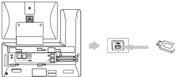
Note: The USB port (on the rear of the phone) can also be used to connect ZIP 450M Expansion Modules or a compatible USB headset.
